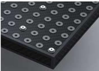
Enhanced version of EC-series. At each mount location a CFRP tube links the top and bottom shell. The CFRP tubes allow easy cleaning of the board, to install removeable additional mounts at the bottom side and to tune the natural frequencies and vibrational damping by inserting adaptive elements.
