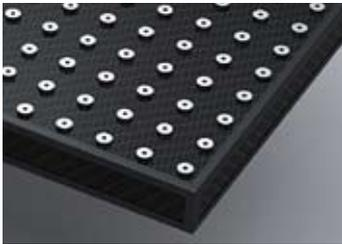
Cost effective series of breadboards based on honeycomb panels with various core materials. Stiffness and thermal stability can be increased by bonding additional CFRP plates on top/bottom side of the board.
