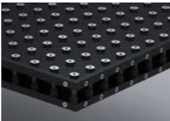
Boards of CA-series are entirely made from carbon fibers. Top and bottom shell consist of several mm thick CFRP shells, structurally joined by tubes made from CFRP. In addition to the advantages of AD-series, boards of CA-series allow the integration of optical/electrical components inside the stiff carbon shell and to route easily wires and optical fibers. Side walls can be installed removeable.
