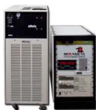
Thermal Support Subsystem & Chiller
