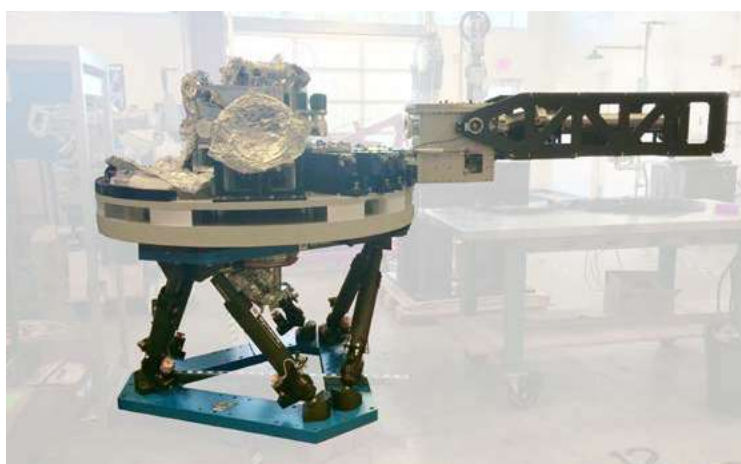
JORAN actuators at LBL are longer to enable a \pm 12.5^\circ rotation around Z. This JORAN hexapod has also been customized to support a 3.2 tons payload.
